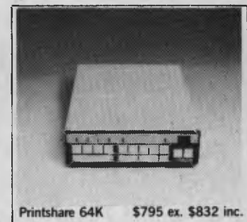
Printshare. Intelligent print buffer. 3 computers to one printer, 2 computers to two printers, one computer to 3 printers. Queues the jobs. Bypass, copy functions.
